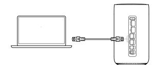
Connect one end of the Ethernet cable to either of these two LAN ports, and the other end to your Laptop or other devices.
